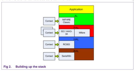
Every component has to be initialized before usage. E.g. Initialization of the BAL layer requires specific context or data parameter to be fed into the component.
